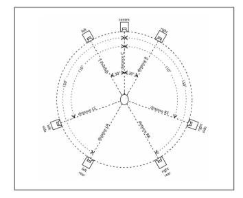
Fig. 3 5.1 and 7.1 Surround Loudspeaker Positioning
