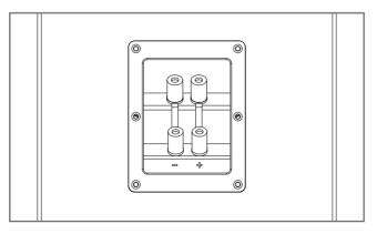
Fig. 4 SCM12 Pro Passive Input Panel
