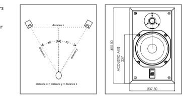
Fig. I Stereo Loudspeaker Positioning
